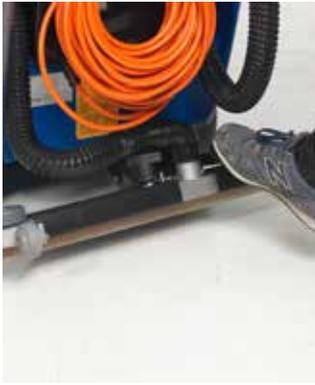
Foot operated squeegee lifting system. The squeegee is placed close to the machine body providing better turn away from walls and improved maneuverability.
